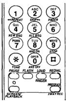
olf the SCREEN/PLAYBACK indicator flashes when you press SCREEN/PLAYBACK, the answering system is off. To turn it on, press [8].
